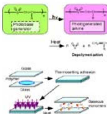
Figure 1: Photoinduced depolymerization of poly(olefin sulfone)s containing photobase generators and a sequence showing a photodetachable thermosetting adhesive.
