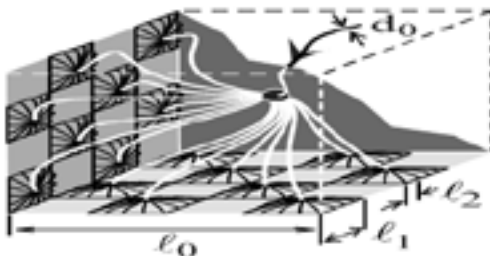
Figure: One cell of parametric material: optic fibers supplies laser pulses of light to optoelectronic switches
